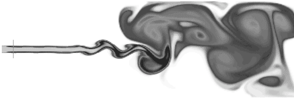
Fig. 2. Shaded contours and cross section plot of mass fraction. Solutions obtained with present high order scheme: a) Unlimited scheme, b) Scheme with FCT-like procedure.
